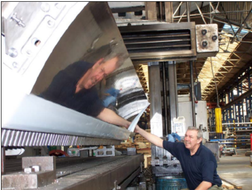
Final Inspection of a Newport Attwood Former Top Lip Assembly.
